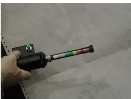
Fig. 3-20: Probe used in BAM feasibility test for crack detection in rivet holes. The depth of the probe (see colours) in the rivet hole is a hint for the depth of the failed member
