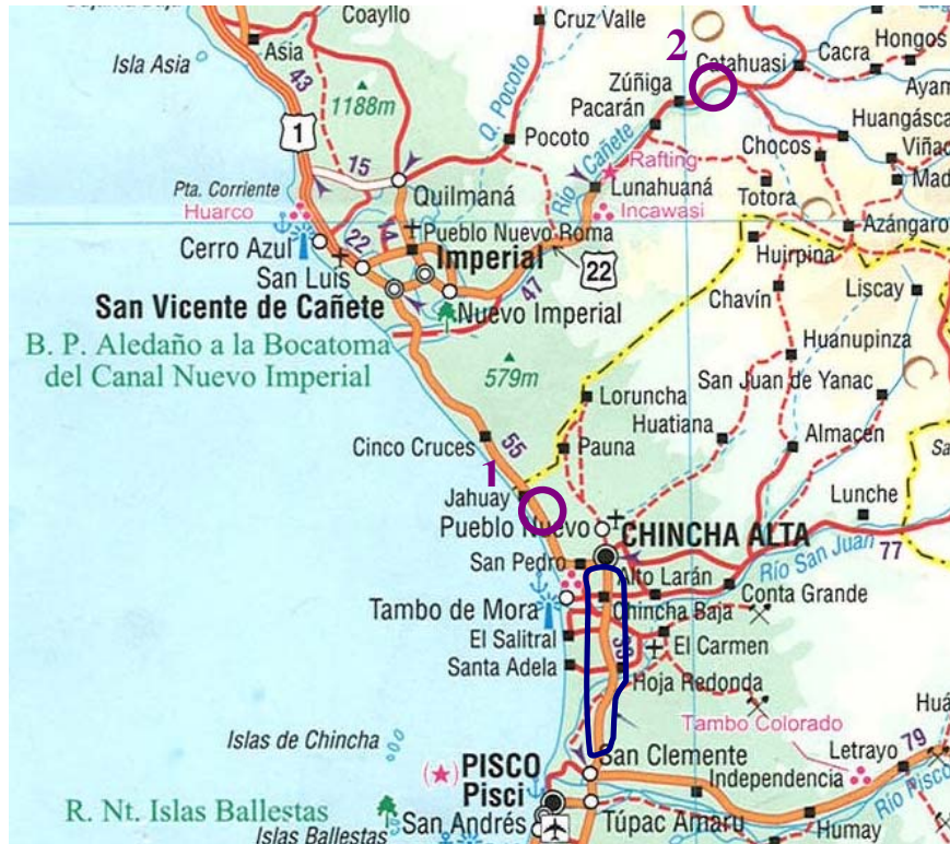
Figure 3.7 Stretch of the Pan-American Highway affected by landslides and soil failure of road structure (delimited in dark blue colour). Points 1 and 2 (violet circles) show the location of landslides observed during the visit.
