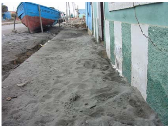
Figure 3.1 Liquefied uniform medium/fine size sand (note undamaged street to the left of the boat)
