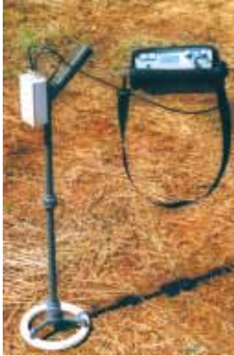
Figure 3.3: A Bartington meter for measuring magnetic ground disturbance. Notice the way that it resembles a conventional metal detector.
