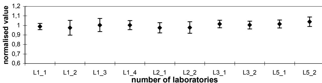
Figure 3-17 - Results of preliminary interlaboratory testing for the model compound benzophenone normalised to the statistically evaluated overall mean of the 10 data sets (Lab x_sample y).
