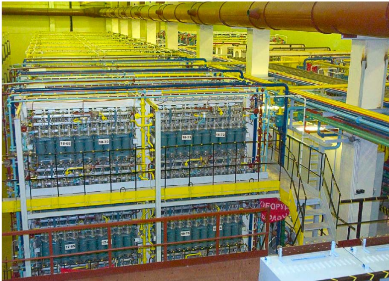
Fig. 9. Cascades of the centrifuges for ^{76}\text{Ge} production at the Svetlana Department.
