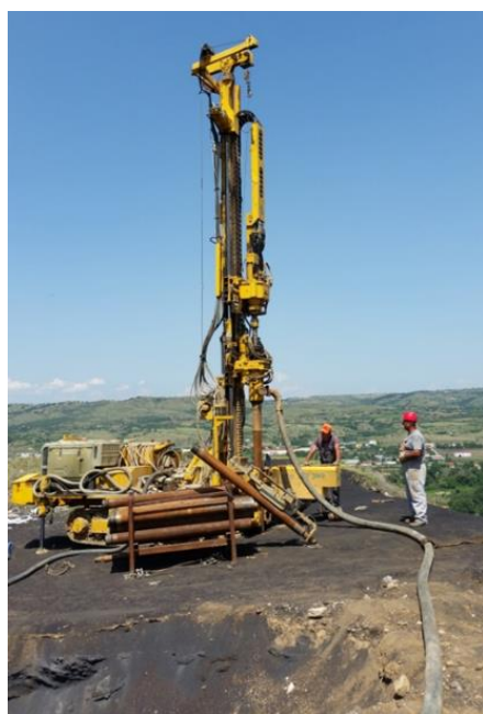
Fig. 4. Air core drilling rigs and in situ sampling method (photo R. Šajn)
