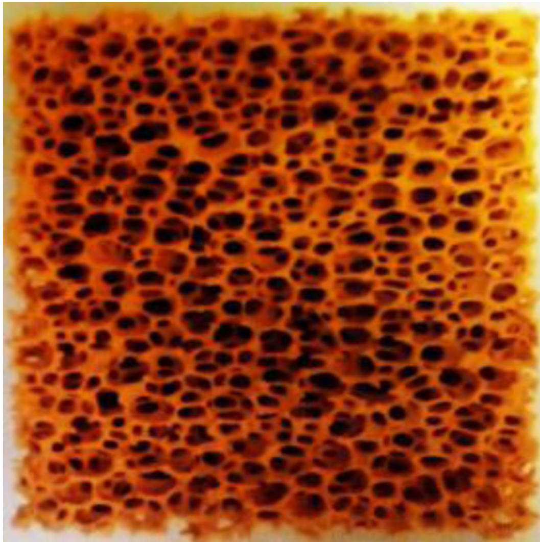
Figure 2. Magnesia-stabilized zirconia 10ppi foam filter (25mm x 100mm x 100mm) used in the experiment.
