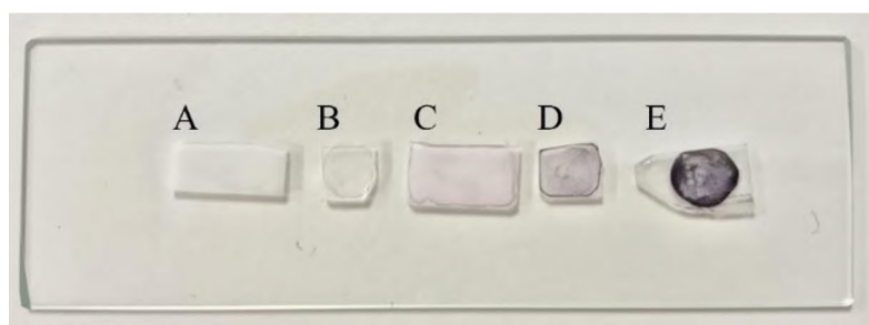
Figure 2. Quartz sample with different AuNP concentrations: (A) no nanoparticles, (B) 1 \times 10^6 nanoparticles per microliter (nps/ \mu\text{L} ), (C) 4 \times 10^6 nps/ \mu\text{L} , (D) 1 \times 10^7 nps/ \mu\text{L} , and (E) 9 \times 10^7 nps/ \mu\text{L} corresponding to a 20 \mu\text{L} -drop of the concentrated suspension ( 1.55 \times 10^{-6} M)
