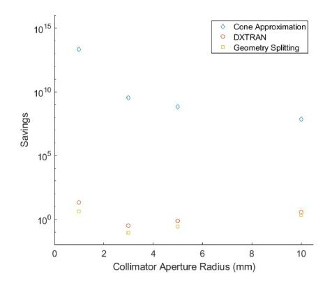
Figure 5: Computational savings for the total tally bin at varying collimator aperture radii
