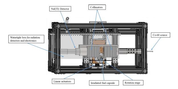
Figure 2.1: Finalized design for a submersible gamma tomography system
