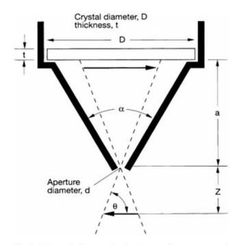
Figure 1.8: Diagram of a Pinhole collimator [32]
