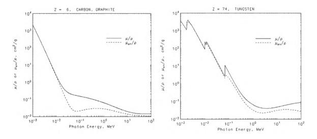
Figure 1.6: Mass attenuation of carbon from 0-20 MeV (Left) and mass attenuation of tungsten from 0-20 MeV (Right) [26]
