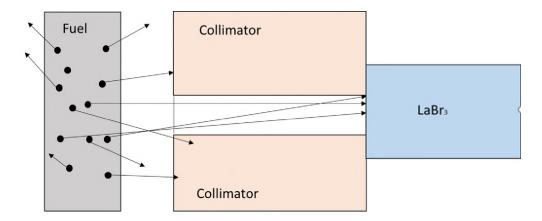
Figure 2.4: Isotropic photon emission from the nuclear fuel to the scintillator detector
