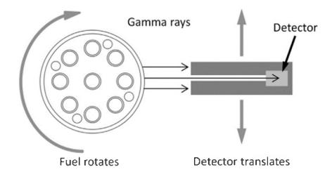
Figure 1.7: Gamma emission tomography system drawing of the Halden Reactor Project system [27]
