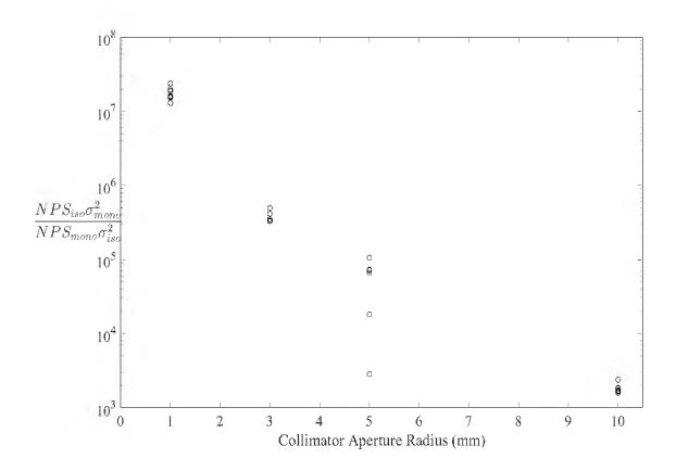
Figure 6: Computational savings of all photopeaks at various collimator aperture radii
