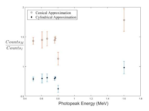
Figure 4: Ratio of the photopeak areas for each transport method for seven high intensity photopeaks at their corresponding decay energies. The ratios are calculated using both the truncated cone normalization and the cylindrical normalization for a 1 mm aperture collimator
