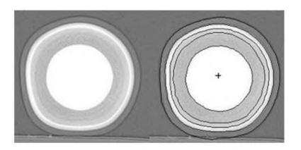
Figure 1.3: X-ray image of a TRISO particle (Left) and an X-ray image of a TRISO particle using PCI (Right) [1], [4]
