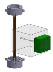
Figure 1: Emission tomography design (not modelled to scale). Gamma rays emitted from the fuel rodlet (cylinder) pass through a tungsten pinhole aperture (grey cube) and into a pixelated array of CZT detectors
