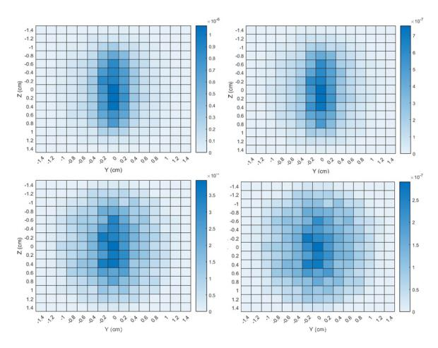
Figure 3.4: Emission probabilities of 8% (upper left), 5% (upper right), 2% (lower left), and 1% (lower right) of Cs-137 at a 0° rotation. Signal is normalized per particle history
