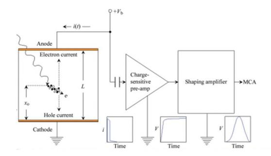
Figure 1.12: Example schematic of a semiconductor planar detection system. Electronhole pairs are created from ionizing radiation directly proportional to the energy deposited [68]
