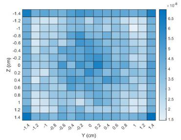
Figure 3.3: Signal per source particle due to scattered photons in each pixel volume
