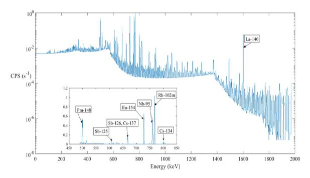
Figure 3: MCNP 6.1 pulse-height tally in the scintillator crystal of the gamma detector
