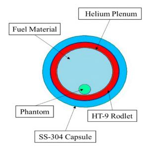
Figure 2.6: Nuclear fuel capsule with a Cs-137 phantom at a 0 ° rotation. 0 ° represents the furthest point within direct line of sight to the detector
