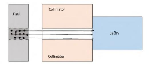
Figure 2.5: Monodirectionally biased beam of photons through the collimator aperture toward the scintillator detector
