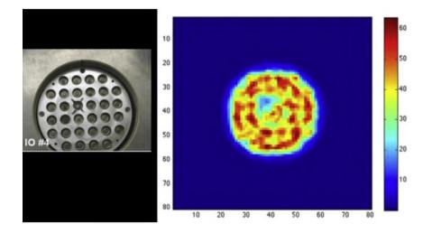
Figure 1.2: Emitted fast neutron tomograph of a MOX fuel assembly with a DU pin marked by an X on left [1], [3]
