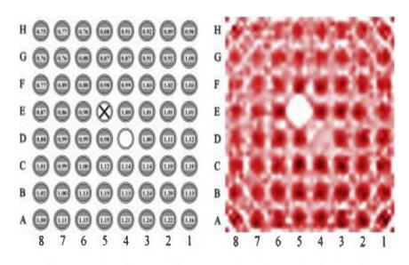
Figure 1.4: Left: Fuel assembly map where the "x" represents a missing rod and the blank circle represents a swapped rod. Right: Cs-137 tomogram and corresponding qualitative fission product concentration in each rod [1]
