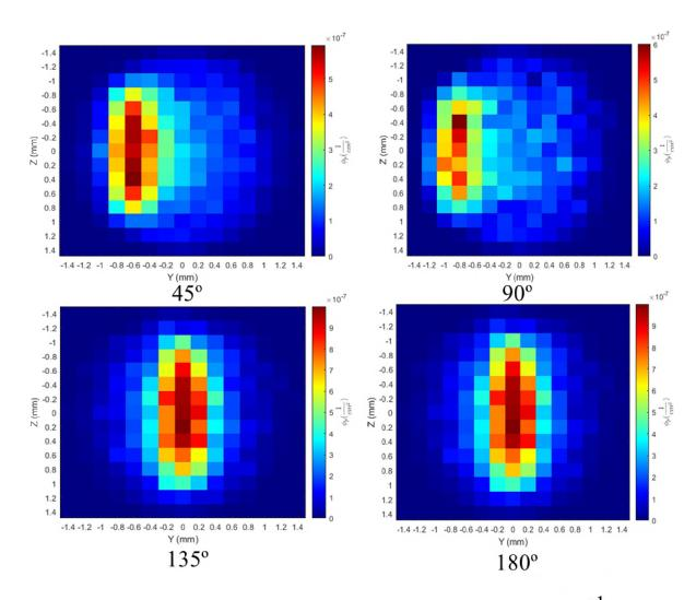
Figure 3.6: Radiographic projections using an MCNP normalized photon flux  $(\frac{1}{cm^2})$  of a Cs-137 phantom at stated angles. 180° represents the closest point for the phantom relative to the detector system
