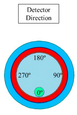
Figure 3.5: 4 rotational angles that establish a relative rotation pattern for the phantom (green cylinder) in 90° increments relative to the detector direction
