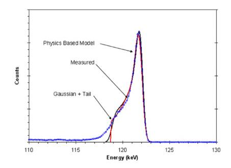
Figure 1.13: Plot comparing a charge carrier trapping model with measured results (blue), a model of charge carrier traping (black), and a fitted gaussian function (red) [86]
