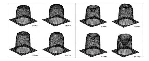
Figure 1.5: (Left) Activity distribution of Eu-154 in UO<sub>2</sub> from 52 GWd/t to 126 GWd/t acquired through gamma emission tomography. (Right) Activity distribution of Cs-137 in UO<sub>2</sub> from 52 GWd/t to 126 GWd/t acquired through gamma emission tomography [20]
