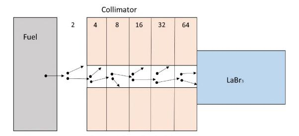
Figure 1: Geometry splitting of the tungsten collimator (not drawn to scale)
