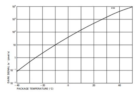
Figure 1.11: Dark Current curve for a CCD97 with respect to temperature [56]
