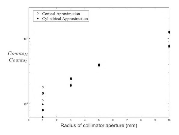
Figure 5: Comparison between of isotropic and monodirectionally biased (post normalization) count rates as a function of aperture radii. Each data marker indicates a photopeak. Ratios for the seven strong photopeaks are shown in each cluster
