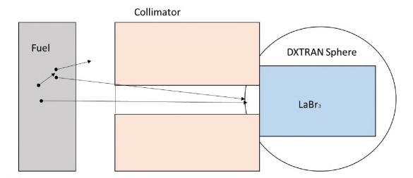
Figure 3: Geometry with a DXTRAN sphere around the detector cell tally region
