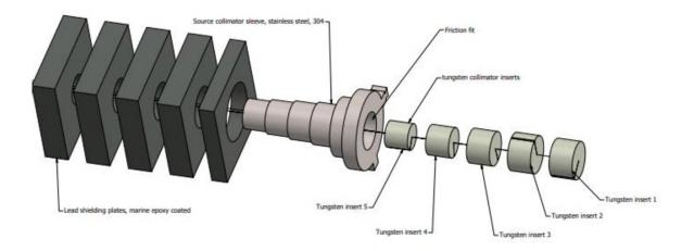
Figure 2.2: Diagram of the source side parallel beam collimator with lead shielding plates, a structural SS304 sleeve, and tungsten inserts
