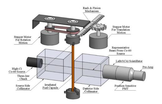
Figure 1: CAD model of the gamma tomography system
