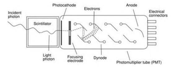
Figure 1.9: Diagram of a generic scintillator
