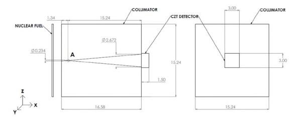
Figure 2.3: Pinhole collimator design combined with a CZT detector
