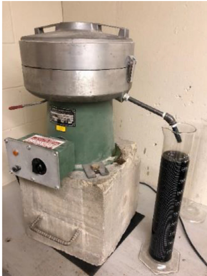
Fig. 2. Centrifuge extraction apparatus: extraction of asphalt-solvent solution.
