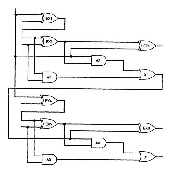
Figure 31. Diagram for the 2 bit adder-subtracter
