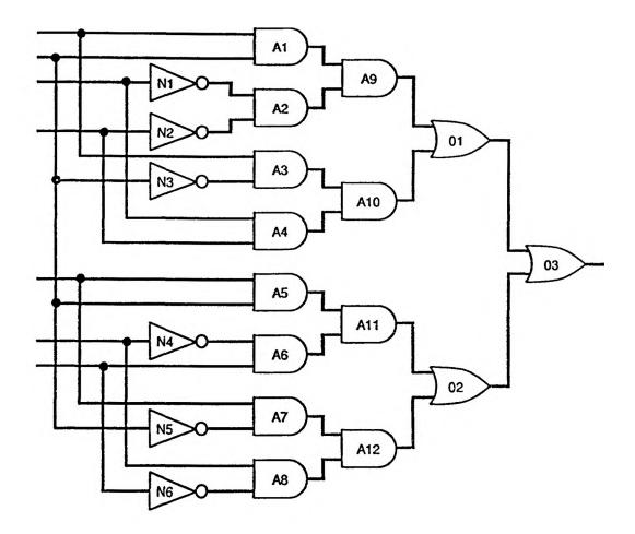
Figure 30. Diagram for an overflow detector
