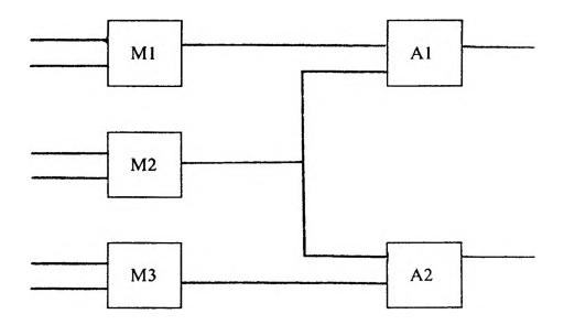
Figure 35. Diagram of an arithmetic circuit
