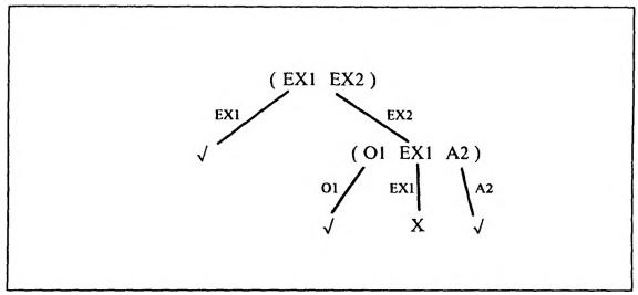
Figure 24. HS-tree for full adder before measurement information
