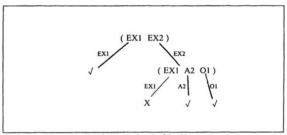
Figure 6. A hitting set tree for diagnosing the full adder
