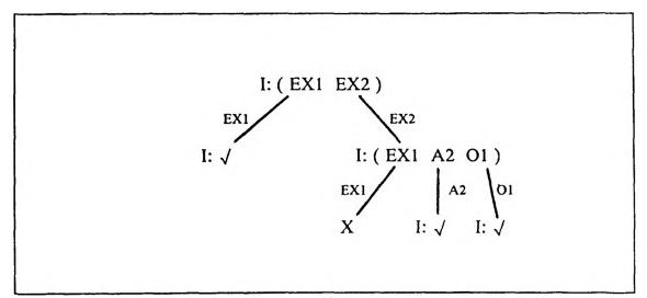
Figure 21. HS-tree for full adder under a single observation set
