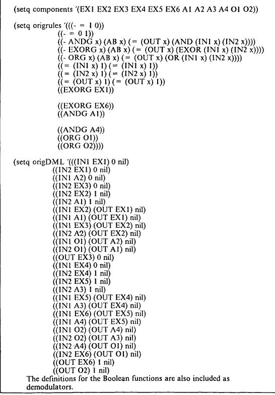
Figure 12. Lisp input to the theorem prover for the two bit adder-subtracter
