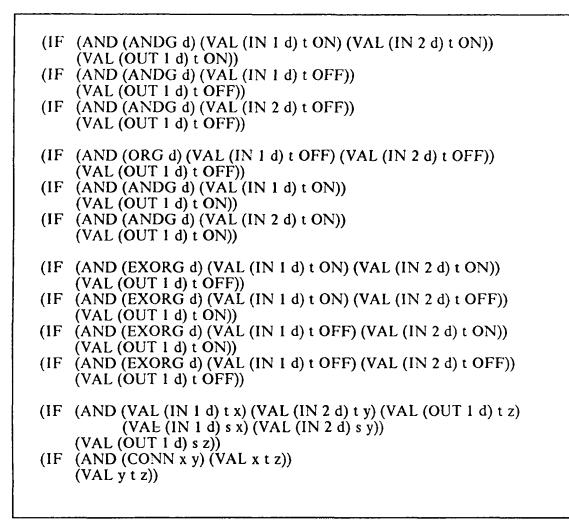
Figure 4. Behavioral description of gates and connections
