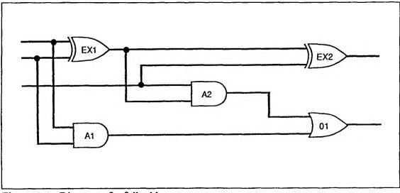
Figure 1. Diagram of a full adder
