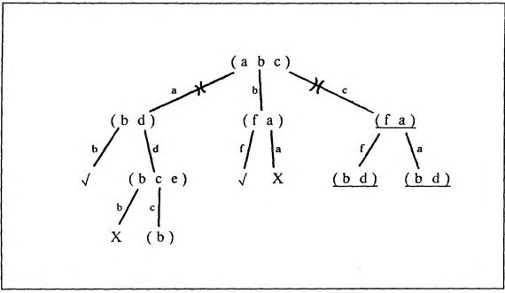
Figure 14. HS-tree with redundant edges marked
