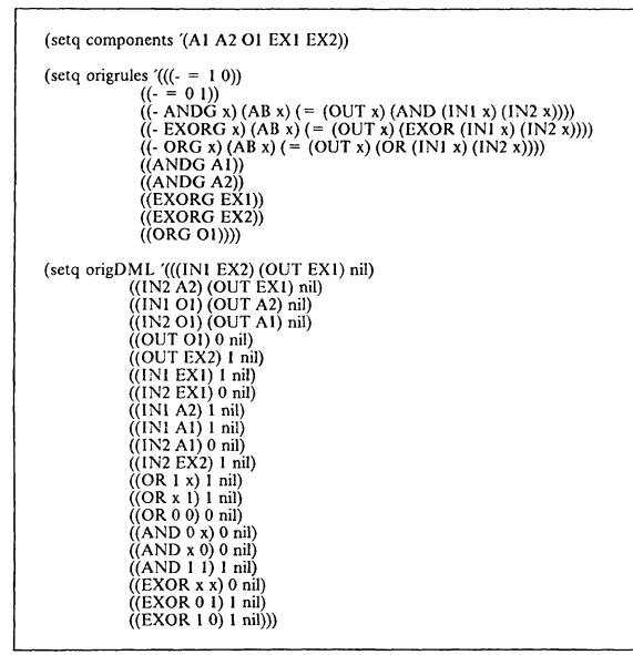
Figure 11. Lisp input to the theorem prover for the full adder
