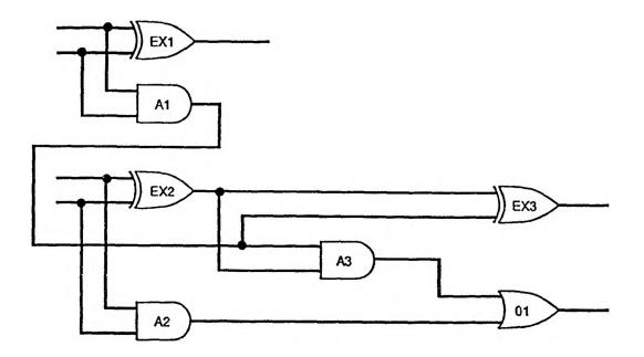
Figure 29. Diagram for the two bit adder
