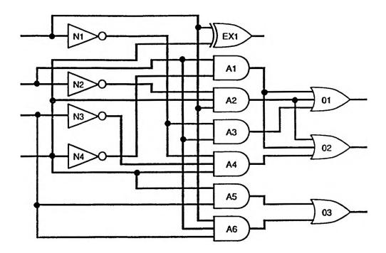
Figure 32. Diagram for a BCD to binary converter
