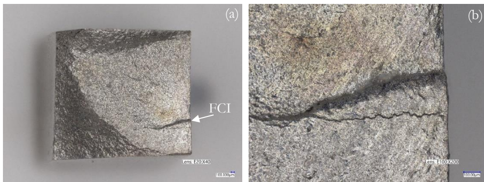
Figure 5: Fracture surface of stress-controlled fatigue test specimen extracted from location #3 of an AZ80 Mg forged component (forged at 300^{\circ}\text{C} , \sigma_{AMP} = 160 MPa, failure after 46,428 cycles) (a) macroscopic view of fracture surface and (b) detailed view of secondary crack at FCI location.
