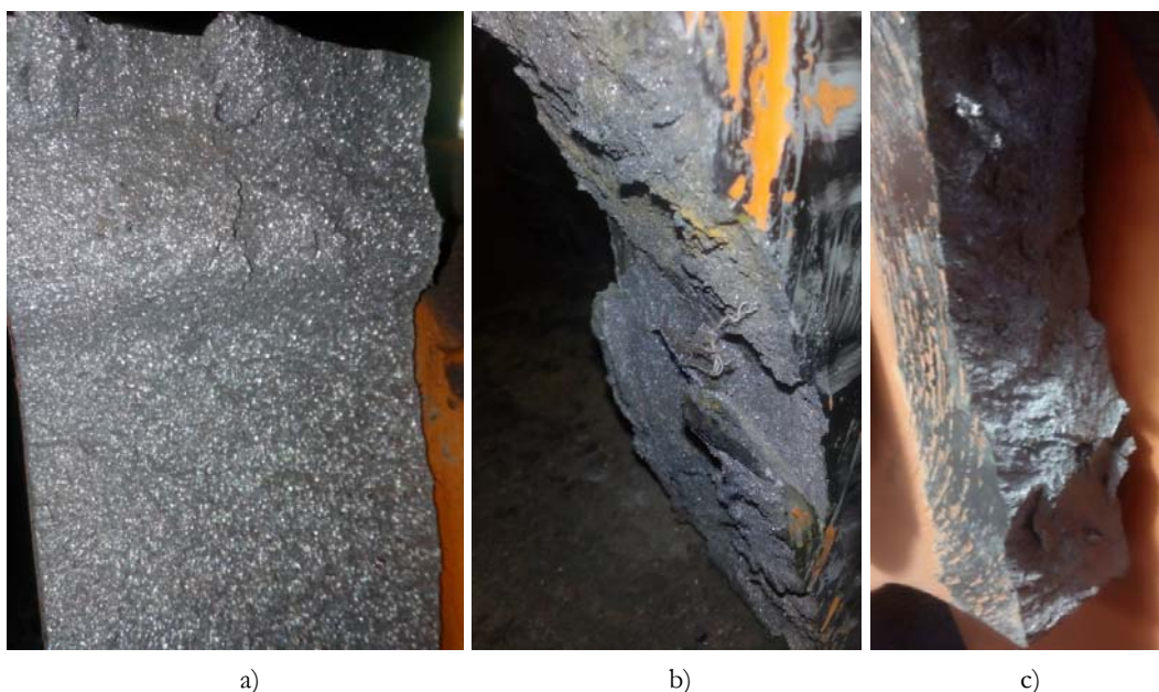
Figure 2: a) Appearance of fracture surfaces of the welded lever; c) fracture surface of the non-welded lever.
