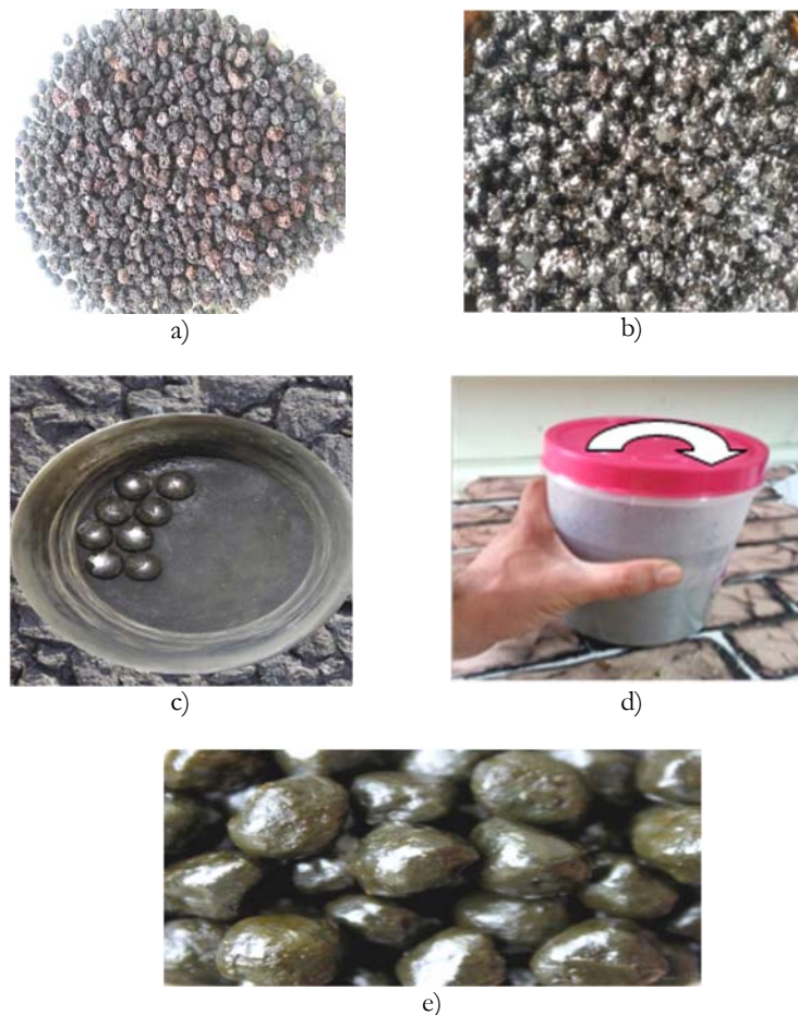
Figure 2: Encapsulation procedure step by step; a) Dry and cleaned porous sands (particle size about 2.3 to 2.8 mm), b) Porous sands with rejuvenator inside the grains, c) Container with a diameter of 2 cm steel balls, d) Energetically circles movement for 15 s, e) The sieved capsules between 3 and 4 mm.
