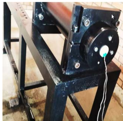
Location of the explosive charge and electric detonator
