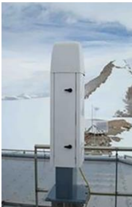
Figure 11. Image of the Vaisala CL31 ceilometer at Princess Elisabeth station in Eastern Antarctica. Figure adapted from Gossart et al. (2017).
