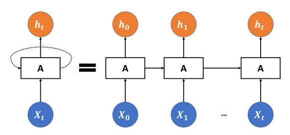
Figure 3.4: The structure of Recurrent Neural Network(RNN).
