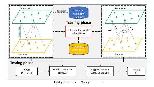
Figure 5.1: The architecture of symptom suggestion method based on weights and ontology
