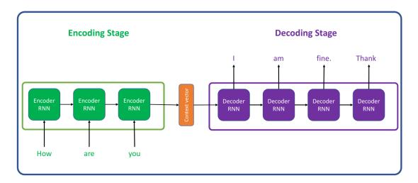
Figure 3.5: Encoder-Decoder architecture (Seq2seq model).
