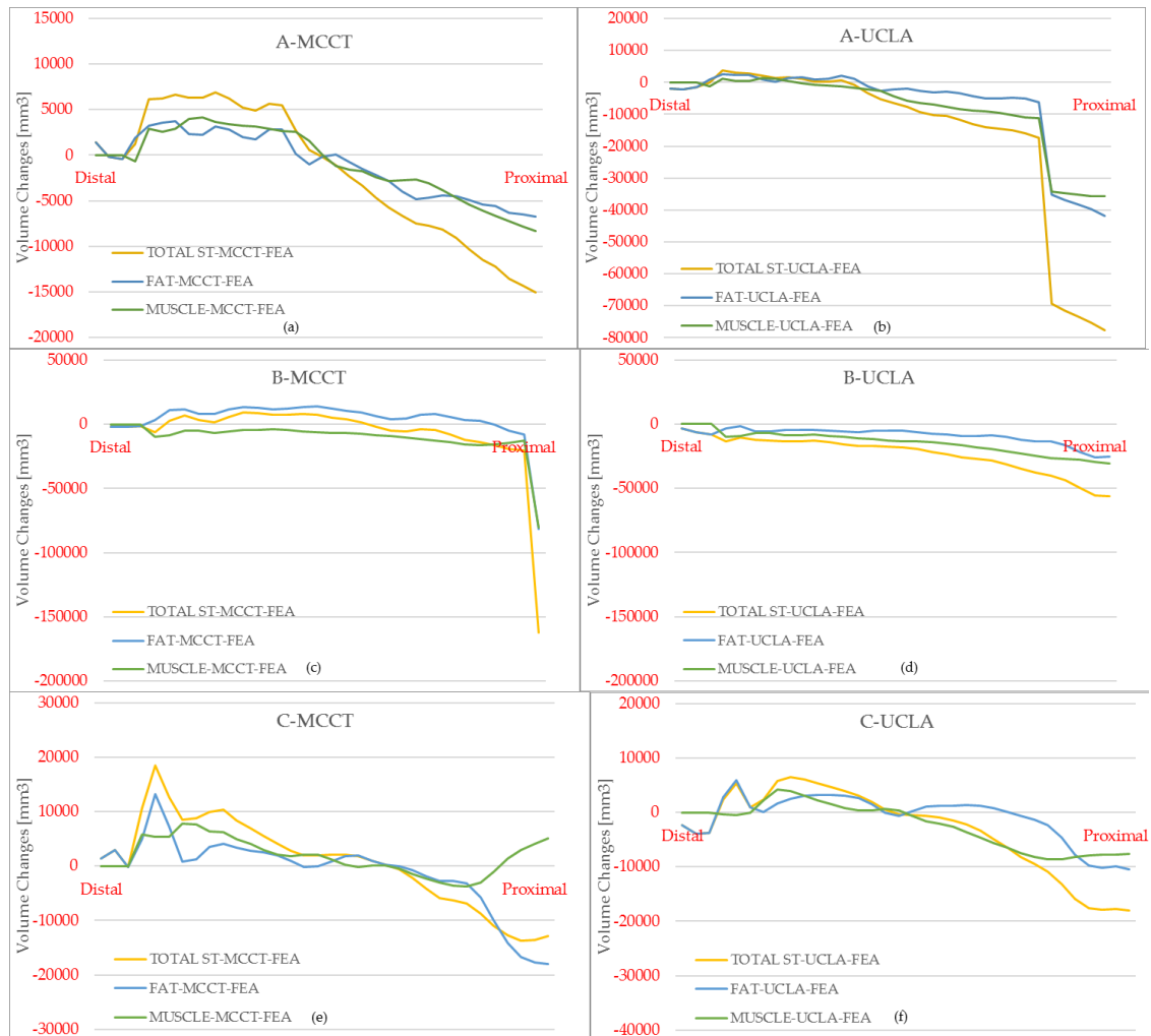
Figure 6.10 Variations of the volumes of deformed soft tissue for total soft tissue, fat and muscle. (a) Results for subject A with the MCCT socket. (b) Results for subject A with the UCLA socket. (c) Results for subject B with the MCCT socket. (d) Results for subject B with the UCLA socket. (e) Results for subject C with the MCCT socket. (f) Results for subject C with the UCLA socket.
