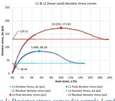
Figure 1: Deviator stress curves for sample 1 and 2
