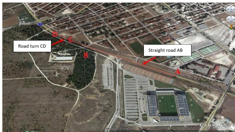
Figure 3: Sequential data of the “straight-curve” study for the calculation of the V_{85i} and the V_{85+i} on road section III (source: Google Earth)
