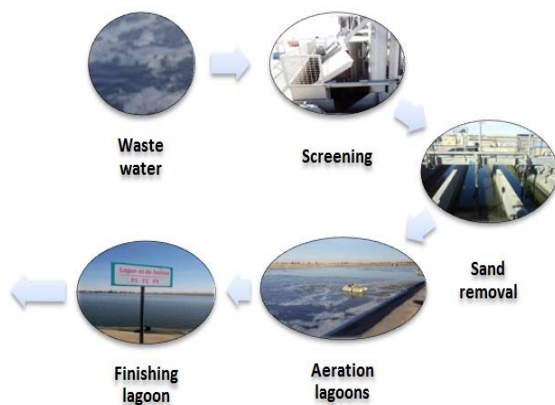
Figure 2. Operating principle of purification Station
