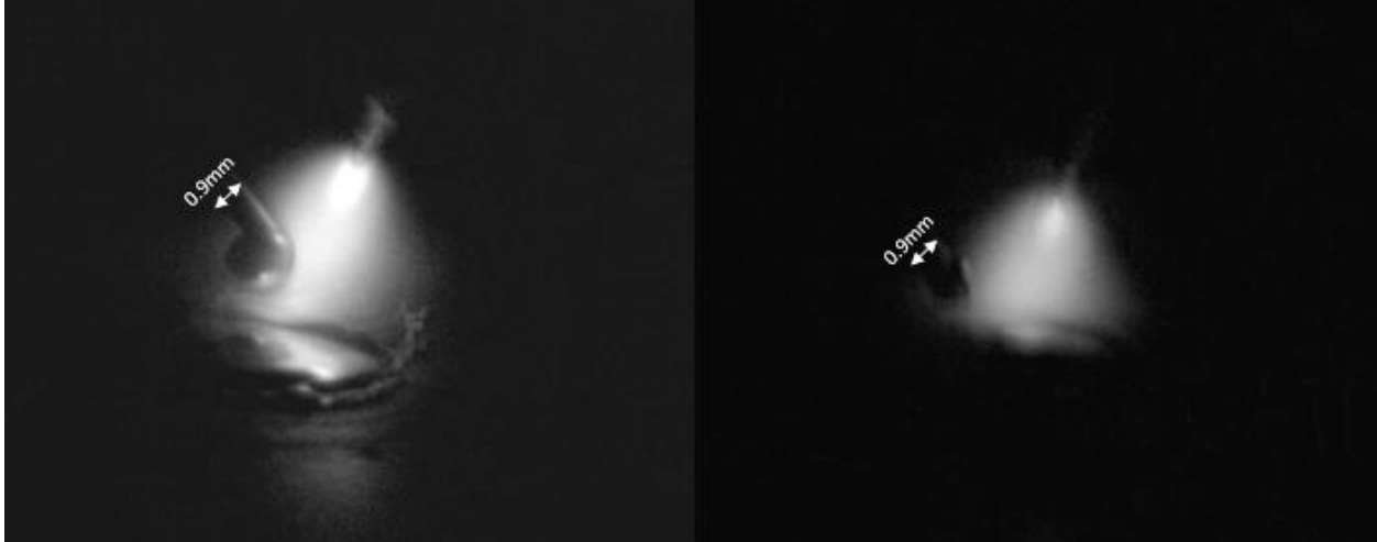
Figure 11. Comparison of 100% argon arc (left) and 3% nitrogen-97% argon shielding gas arc (right).
