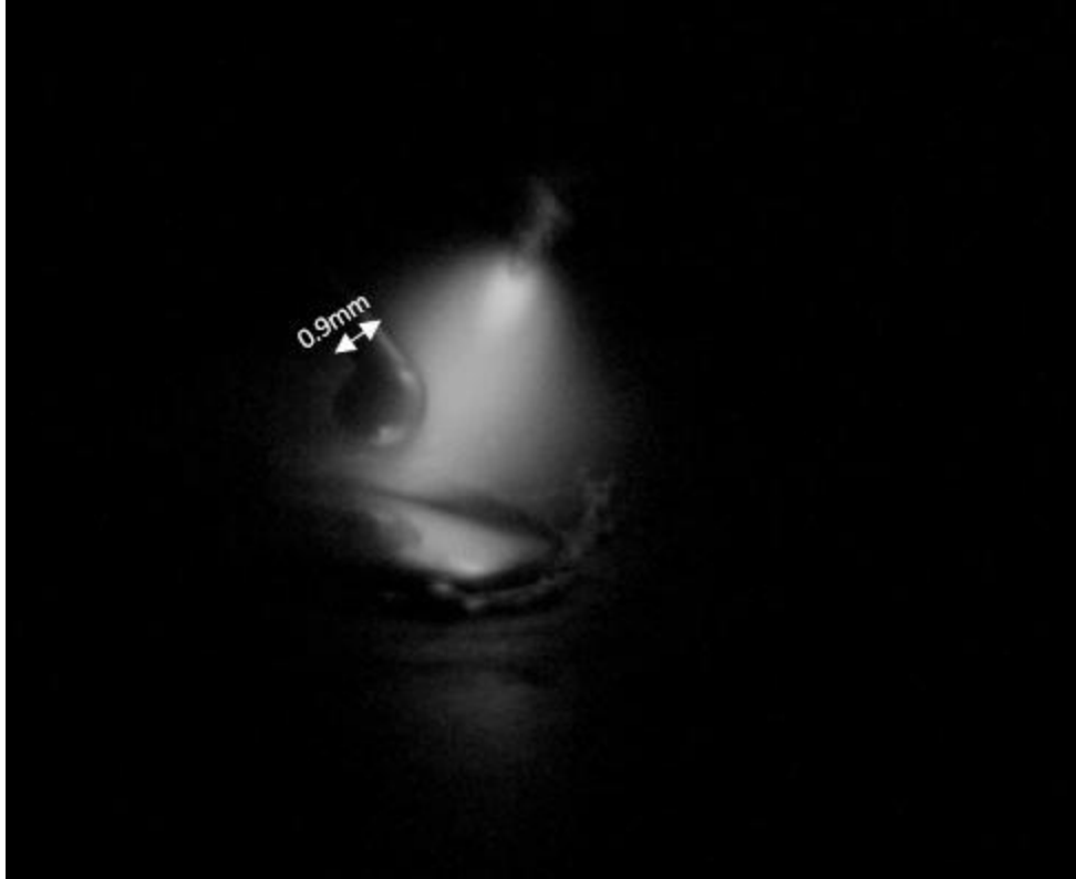
Figure 10. Tungsten arc with the known diameter of filler wire (0.9 mm).
