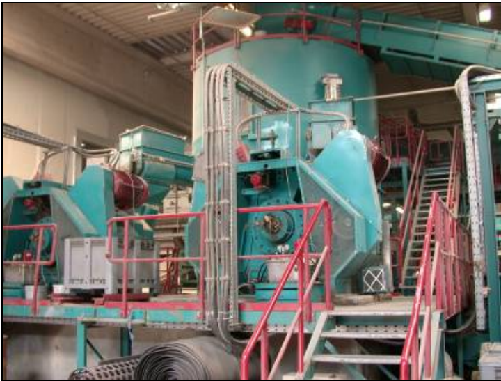
Figure 9: REMONDIS device for SRF production
