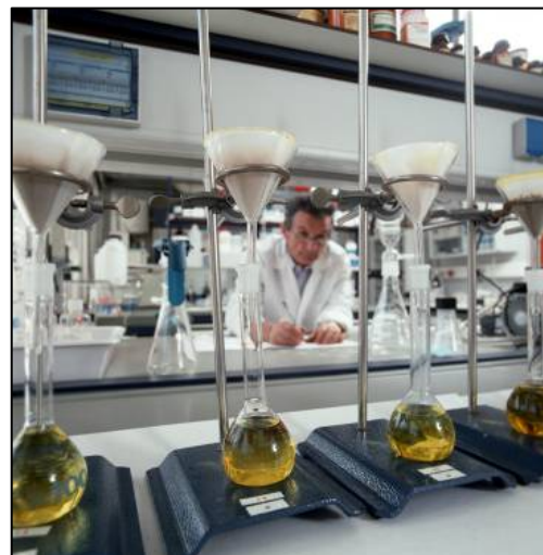
Figure 13: Production of Acidic Digest from SRF by open-vessel digestion under reflux condition
