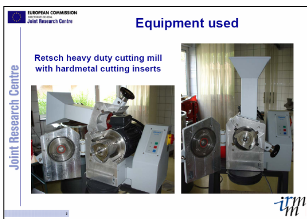
Figure 14: Equipment used for the processing of the SRFs
