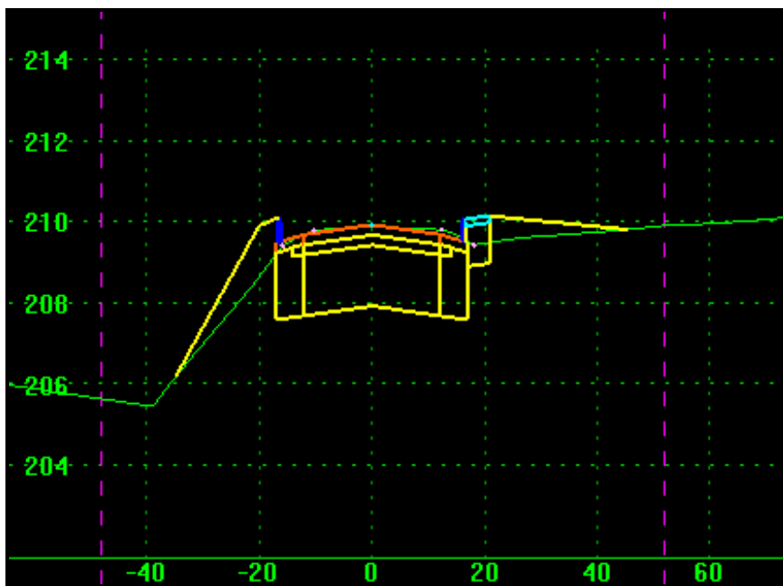
Figure 16-10 Cross Section view with ROW lines displayed.
