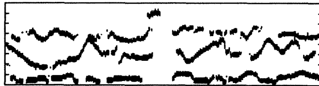
Figure 4. Schematic representation of sinusoidal sentence replicas. Top panel: Four sinusoids are used to replicate the sentence, "The beauty of the view stunned the young boy"; there is one tone for each of the three lowest formants, including bursts, aspirations, and nasals and a fourth tone for the fricative formant. Second panel: The second formant tone pattern isolated from the sentence replica. Third panel: The pattern of the second formant tone time reversed (reflected temporally). Bottom panel: The pattern formed by the tonal replica lacking a second formant analog combined with a temporally reflected second formant tone.
