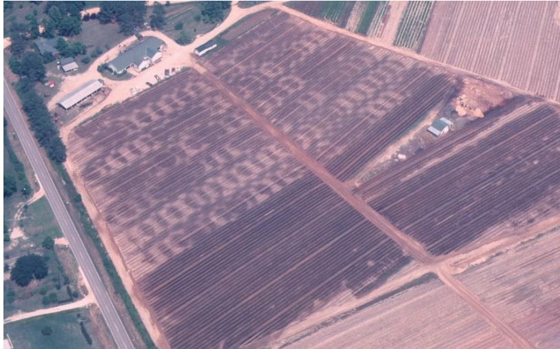
Figure 3. Irrigation pattern from a solid-set irrigation system (12.2 m x 17.7 m) at Opelika, Alabama.
