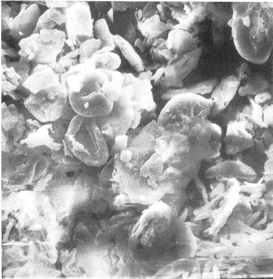
Fig. 4. SEM of sporinite macerals as separated by DGC from the Brazil Block paper coal. The field-of-view is \approx 110 \mu\text{m} wide.
