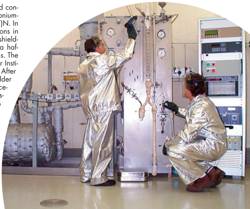
Figure 43 - Sodium filling of the CONFIRM irradiation
