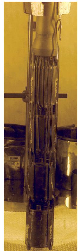
Figure 36 - The as-irradiated stack of four subsized blanket modules with containments and instrumentation prior to dismantling.
