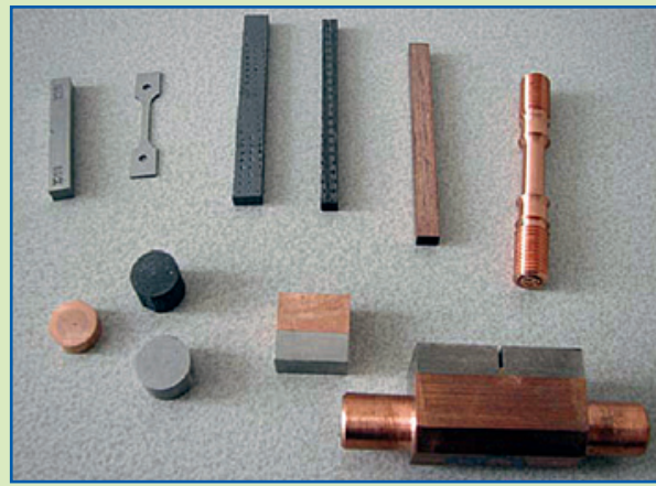
Figure 40 - Typical test specimens of carbon, silicon carbide, tungsten, fiber reinforced copper, and miniaturized divertor elements, from various ExtreMat project partners, before irradiation at different temperature and dose levels
