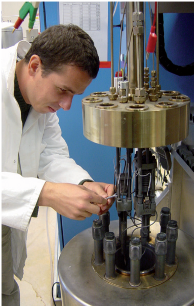
Figure 14 - AMALIA Autoclave for Stress Corrosion Cracking (SCC)
