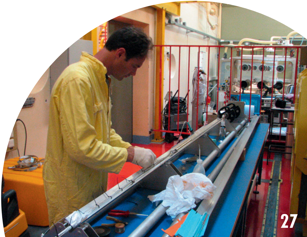
Figure 34 - Assembly of the experiment for graphite irradiation
