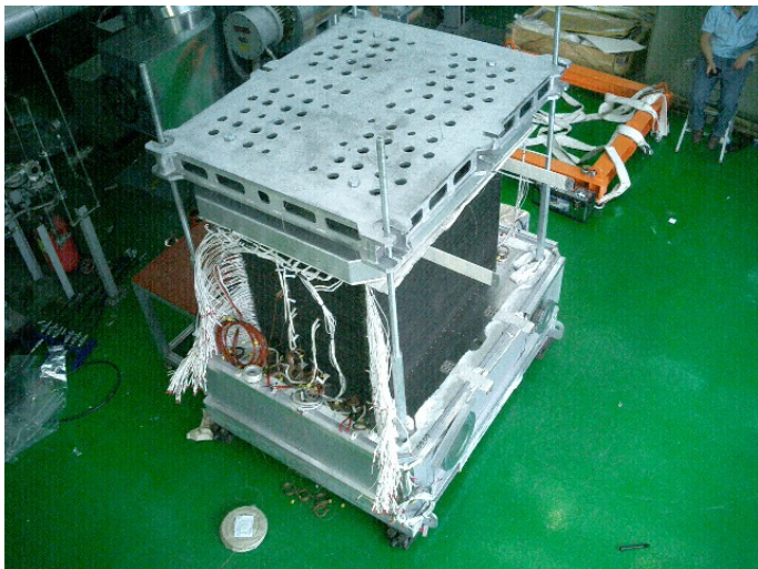
Figure 6. 75 kW test stack for the development of the 250 kW system at KEPCO
