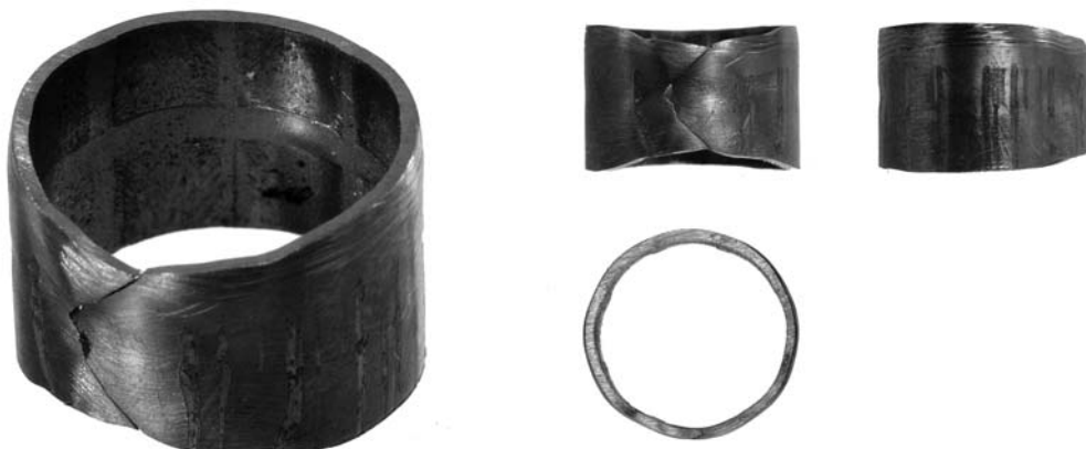
Figure 10: 3D, front, left and top overview of tested Zyr4A specimen. Crack together with local deformation is present. Mandrel test device pattern is visible inside of specimen.
