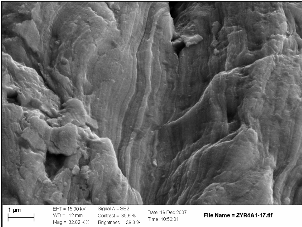
Figure 17 One of the detailed views on the surface deformed zone – shear bands. Picture is presented on the same planes effecting from deformation of specimen.
