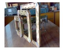
Fig. 3. Reconfigurable multi-beam SWA
