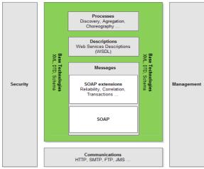
Fig. 2 Web service architecture stack.
