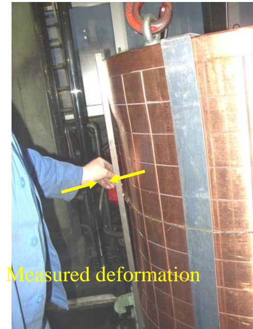
Figure 7: Manual measurement of residual deformation fo Mock-up 1 after p_{max} = 130 MPa
