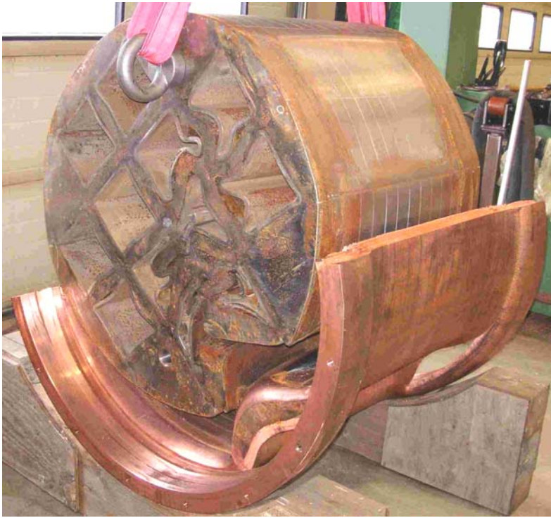
Figure 9: Mock-up 2 after the pressure test
