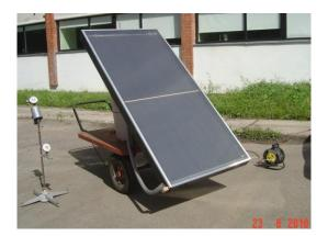
*Fig.5.* Mobile stand for solar collectors' experimental investigation (look from the outside)
