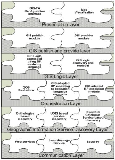
Fig. 2. Multilayered architecture of GIS-FA
