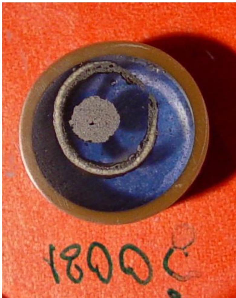
Fig. 22. Cross section of the short fuel rod from test No. 22
