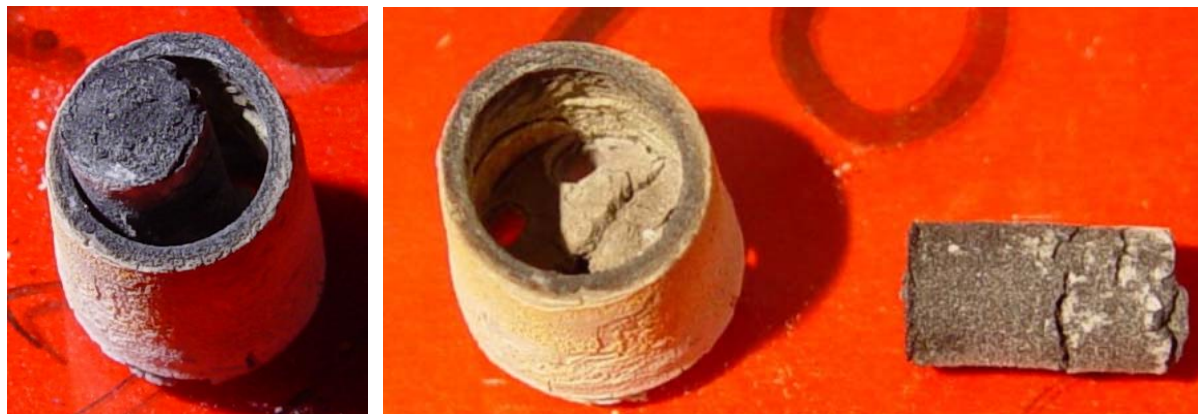
Fig. 16. Short fuel rod sample after test No. 20b
