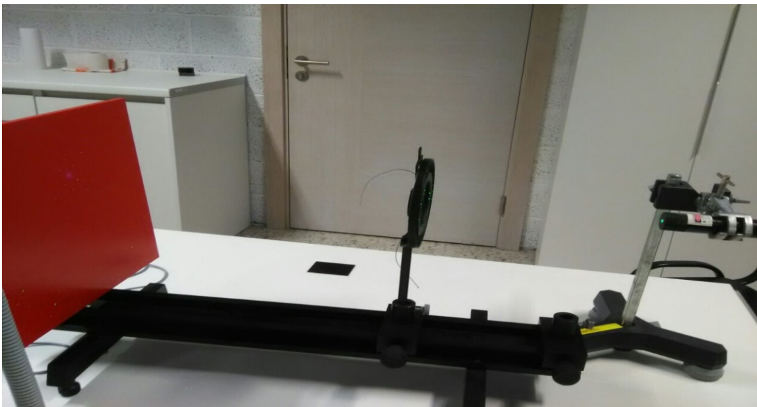
Figure 5 Basic parts of the experimental set: the laser source (right), thin threads (middle) and the screen (left)
