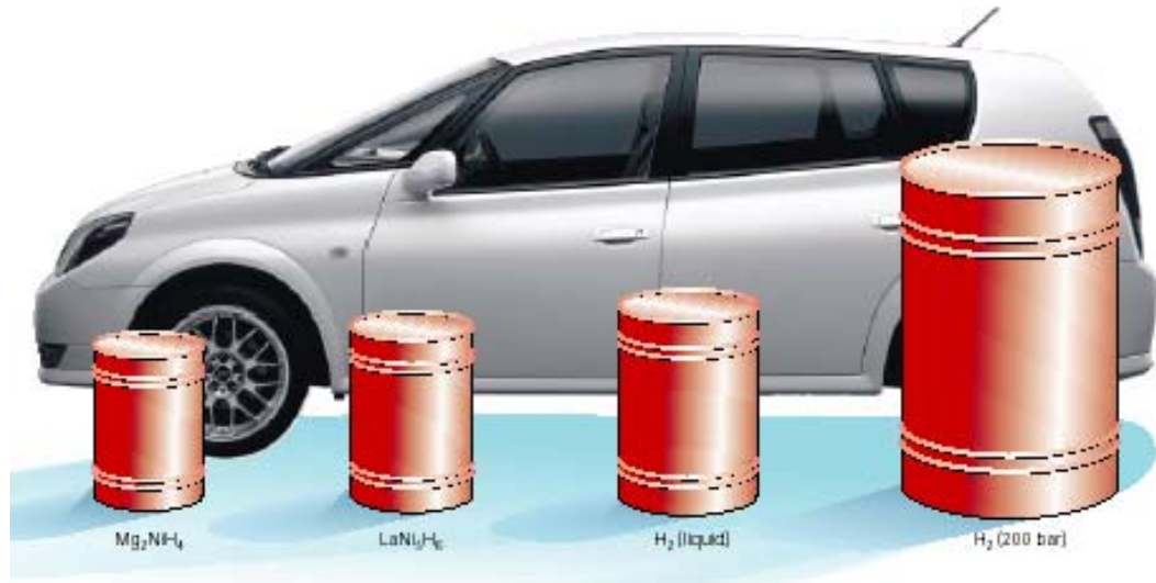
Figure 21 – Volume of 4 kg of hydrogen (needed to run an electric car with a fuel cell) compacted in different ways as schematically illustrated here; size relative to car size [28]
