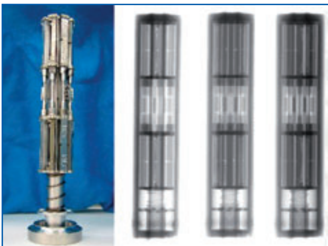
Figure 51 - Assembly of specimens inside IBIS capsule, röntgen image of the three IBIS capsules (300, 500 and capsule for cold testing) before filling with LBE
