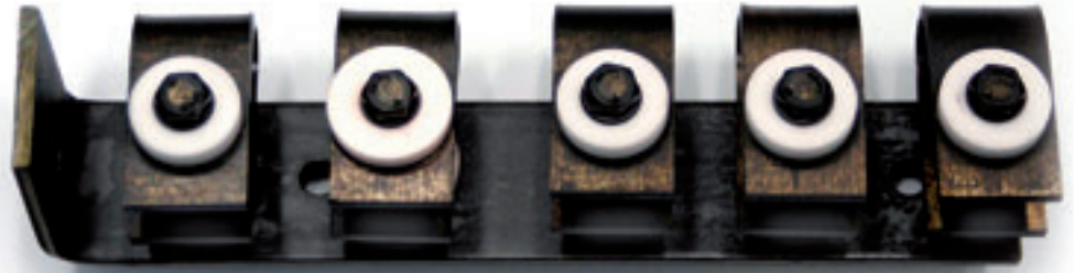
Figure 8 - Typical U-band samples for Stress Corrosion Cracking (SCC)
