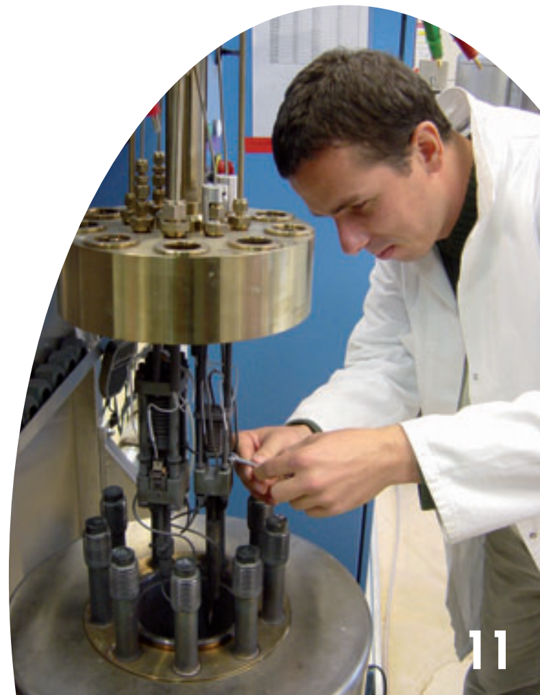
Figure 11 - Autoclave for Stress Corrosion Cracking (SCC)
