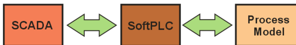
Fig.8 The computer provided with SCADA and PC-based controller interoperable with a physical model of the facility
