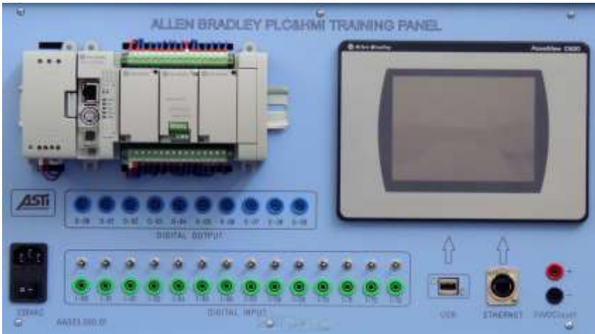
Fig.6. PLC Trainer by ASTI (ASTI, 2017)
