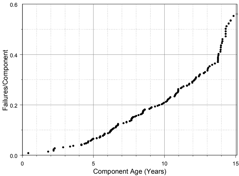
T-A failures -- critical, non-CCF
