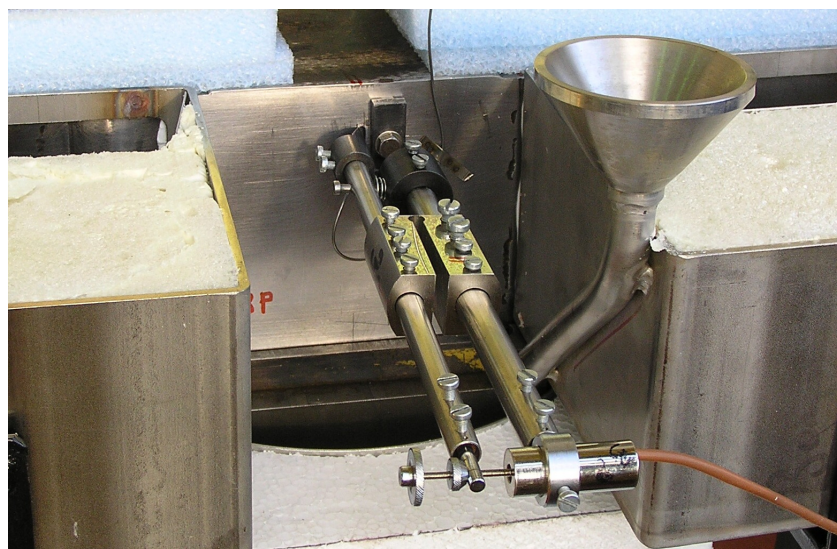
Figure 10 The device for CMOD measurement mounted on the flank of a specimen.
