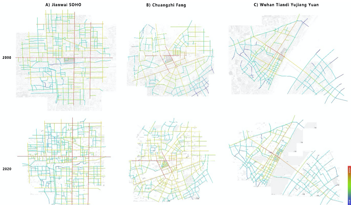
Figure 3 Integration [HH] Analyses of Jianwai SOHO, Chuangzhi Fang and Wuhan Tiandi Yujiang Yuan in 2000 and 2020
