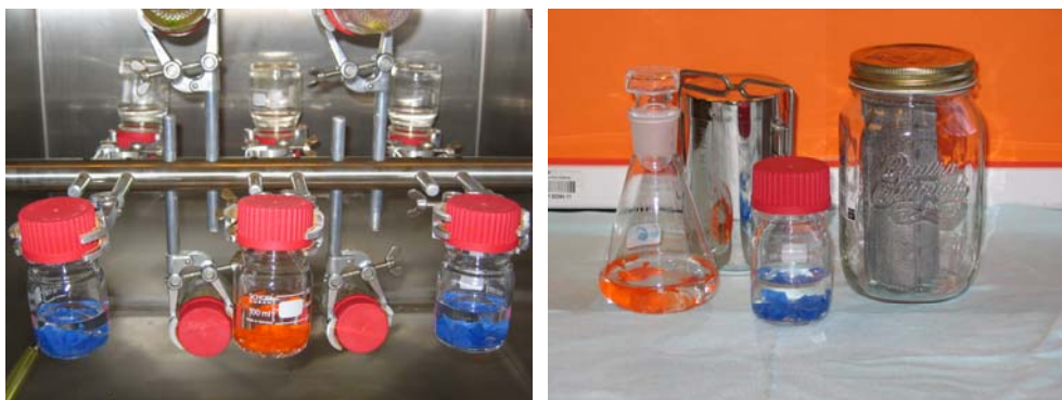
Picture 3: a) Head Over Heels equipment; b) sample vessels for the different methods.
