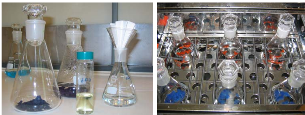
Picture 1: a) Various steps of method EN ISO 14184-1; b) oscillating water bath.
