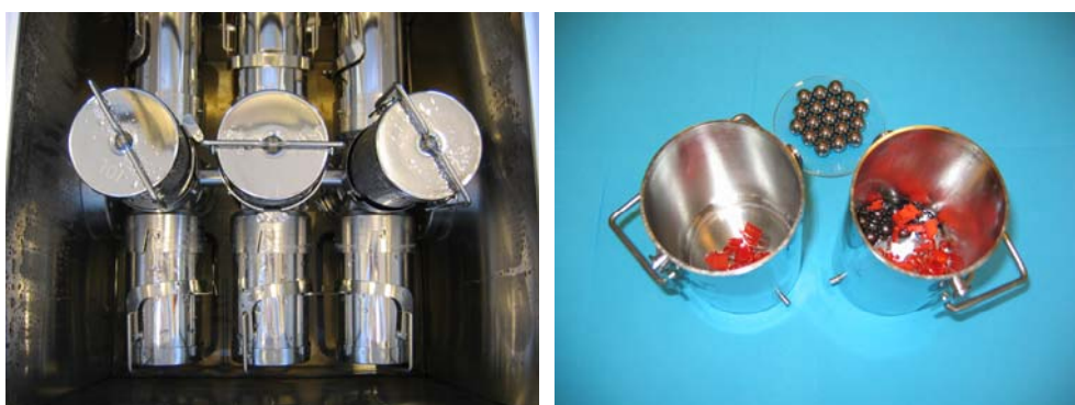
Picture 4: a) Gyrowash apparatus; b) sample vessels for Gyrowash.
