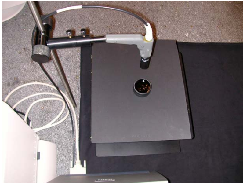
Fig.11 The spectroradiometer ASD-FieldSpec Pro in Reflectance mode
