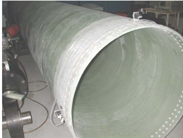
Figure 29 Detail of monolithic tower with accelerometers mounted near the bolt area, for modal analysis in the radial direction.
