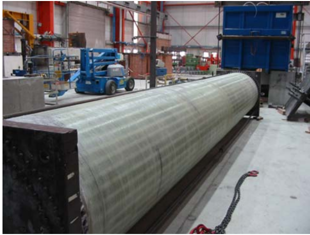
Figure 17 Hybrid tower section with mounted end plates.
