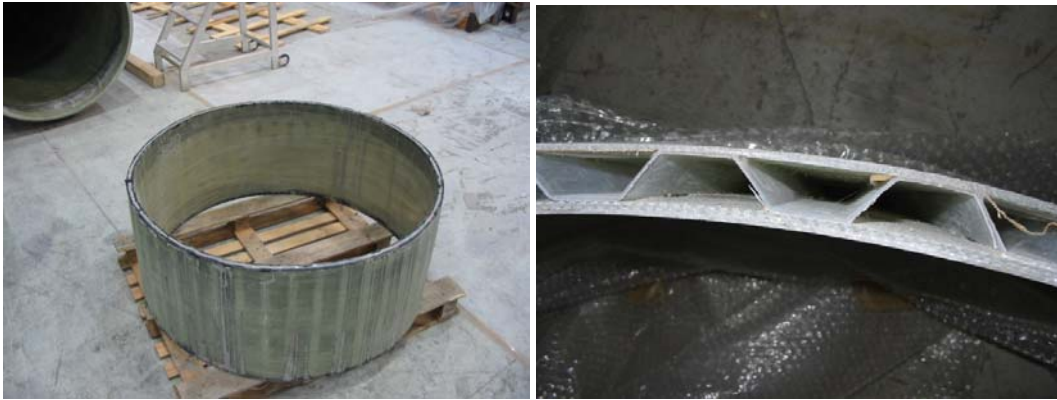
Figure 13 Concrete-filled ring coupon section and detail of empty core. The gap size is 16 mm.
