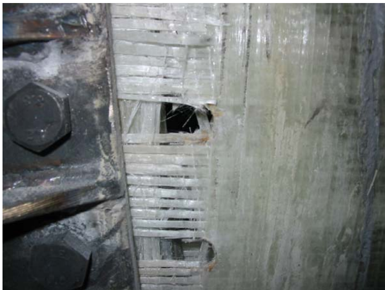
Figure 139 Detail of laminate pull-out area around steel flange
