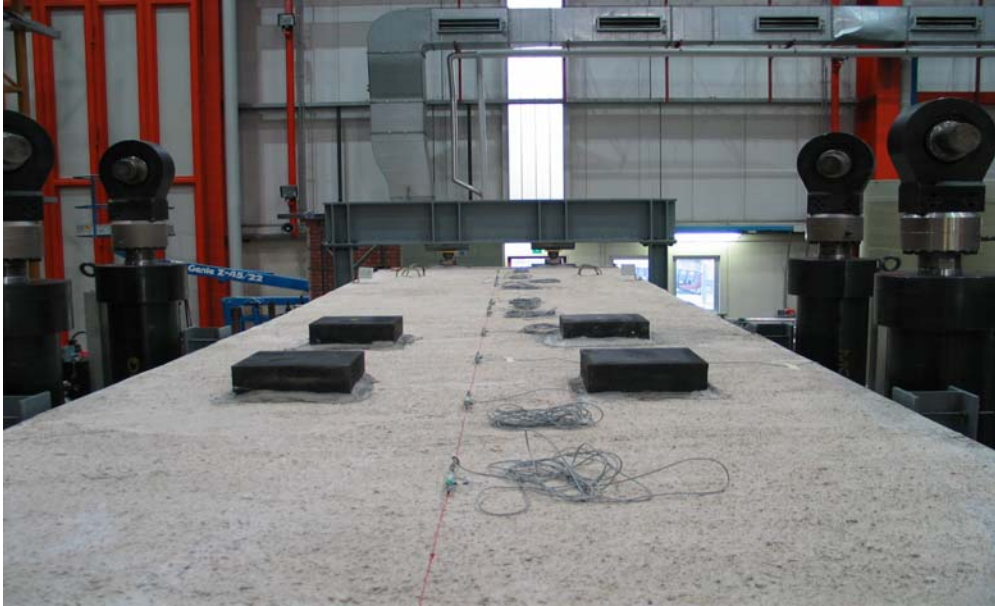
Figure 31 View of loading train steel-rubber bearings.
