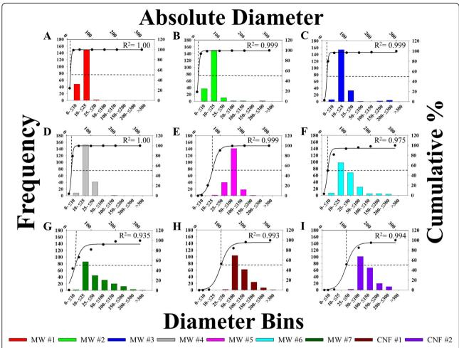
Fig. 3 Distributions of CNT/F diameter. Particles were binned according to size along the lower x-axis with frequency on the left y-axis. Additionally, percentage of accumulation is graphed on the right y-axis with the absolute diameter along the upper x-axis. The overlay line was 3 parameter sigmoidal curve of best fit with the point of 50% accumulation indicated with dotted lines. Sizes are for particles in isopropanol suspension
