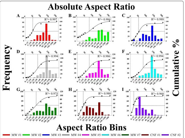
**Fig. 5** Distributions of CNT/F aspect ratio. Particles were binned according to size along the lower x-axis with frequency on the left y-axis. Additionally, percentage of accumulation is graphed on the right y-axis with absolute aspect ratio along the upper x-axis. The overlay line is 3 parameter sigmoidal curve of best fit with the point of 50% accumulation indicated with dotted lines. Sizing was for particles in isopropanol suspension
