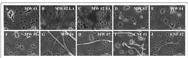
Fig. 2 Representative scanning electron microscopy images of CNT/F in DM to measure two-dimensional agglomerate sizes. LA = large agglomerates and SA = small agglomerates
