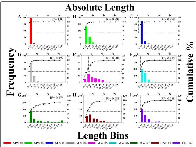
**Fig. 4** Distributions of CNT/F length. Particles were binned according to size along the lower x-axis with frequency on the left y-axis. Additionally, percentage of accumulation is graphed on the right y-axis with absolute length along the upper x-axis. The overlay line is 3 parameter sigmoidal curve of best fit with the point of 50% accumulation indicated with dotted lines. Sizing was for particles in isopropanol suspension
