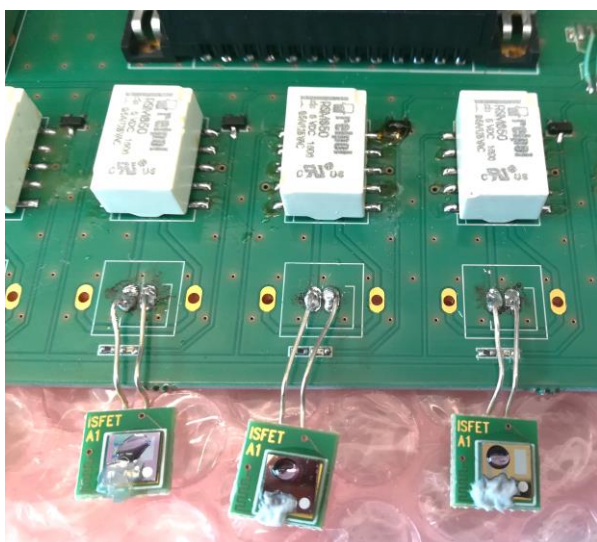
Fig 7. ISFET transistors with applied biological substance
