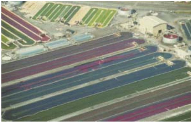
Figure 31: A 90 acre microalgae production facility in Hawaii. The algae grow consuming CO 2 captured from a nearby power plant [95].
